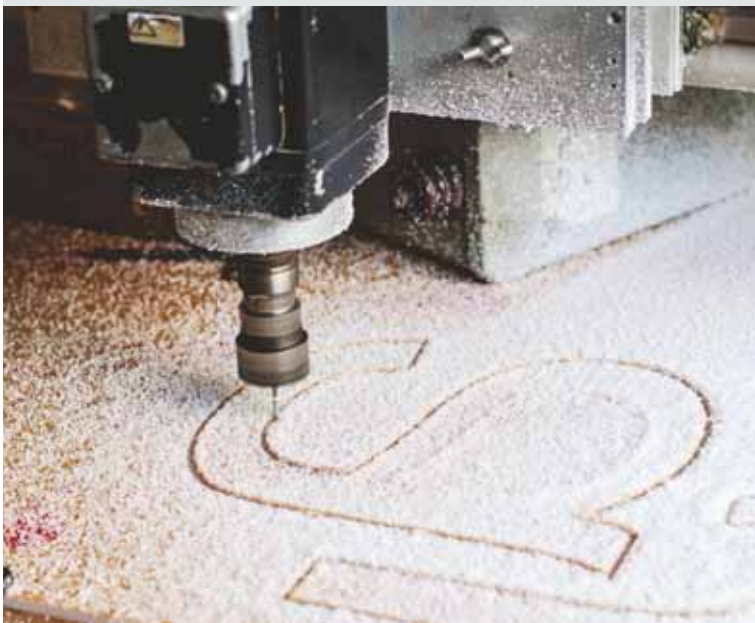
CNC router to cut heavy guage sheets on accurate line drawings.
